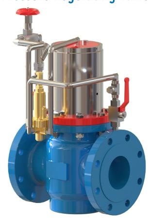
The pilot releases pressure from the valve to compartment at an adjustable rate. By adjusting the adjustment screw, the downstream control pressure can be adjusted to the desired downstream pressure. The pilot will ensure that the downstream pressure will remain stable, even if the upstream pressure changes with demand changes.
